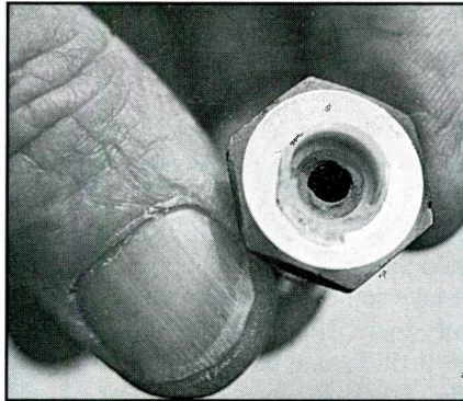
The stud breaks out of the base. Actually, it pulls out from the base!
